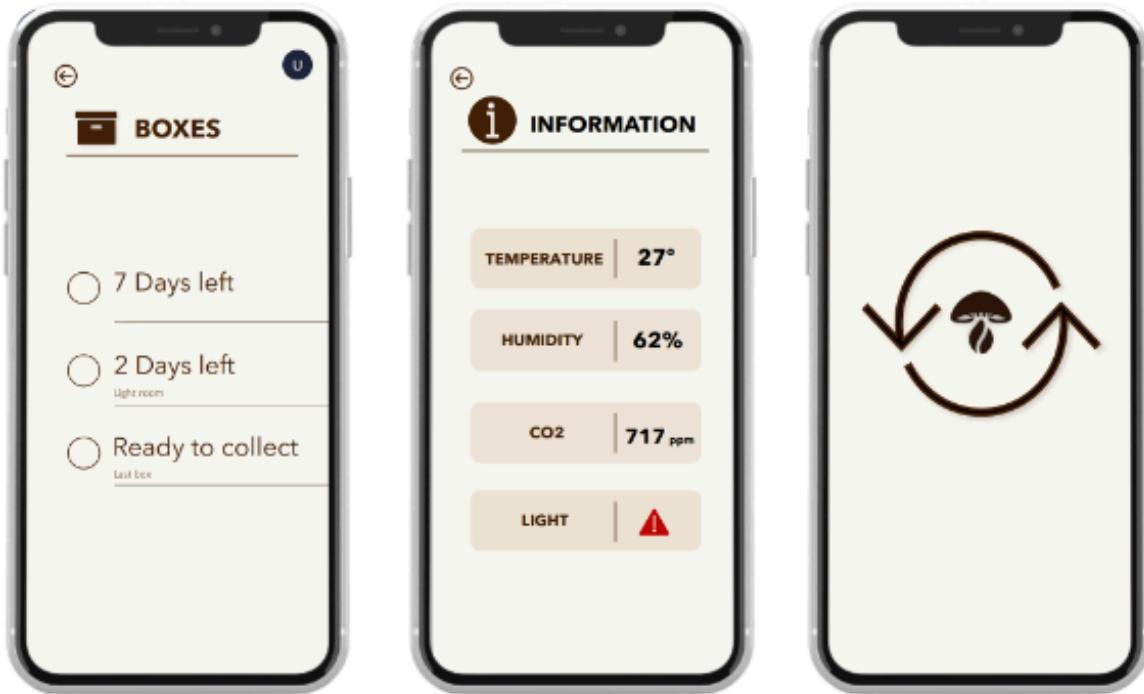
The application will also send notifications in case the mushrooms are ready (as shown in the first screen); and also in case it is necessary to regulate any condition of the composter, (as can be seen in the second screen).
